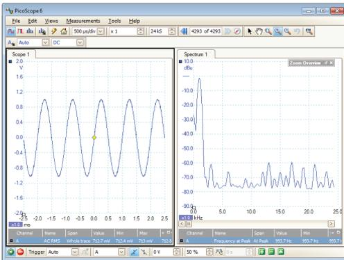
The PicoScope 2104 and 2105 PC Oscilloscopes are connected to and powered entirely by the USB port of a PC or laptop. The market-leading PicoScope software supplied with the oscilloscopes enables analysis of voltage waveforms, includes automatic measurements such as frequency, duty cycle and rise time, and has a variety of trigger settings. It allows the PicoScope 2104 and 2105 to be used as:
